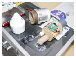
All parts are tethered together with 80-lb Kevlar cord and a multi-strand of crepe paper streamer for it to fall with.
