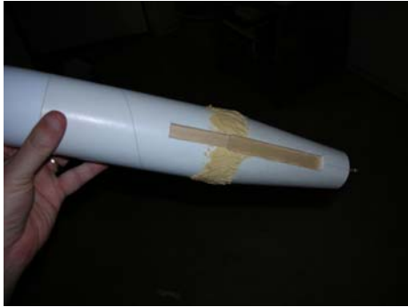
The pre-sanded completed body tube / tail cone.
