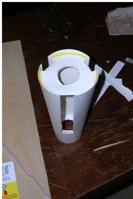
Slots cut in the tail cone.
