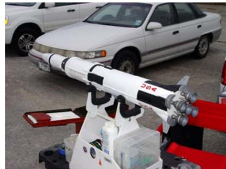
E9 to find out the mount was made for a shorter, kits original choice, motor length. Taped for friction fit of all motors with 1/4 inch tape thrust rings and taped the center motor to the motor retaining hook for added insurance. The launch lug is not 1/4
